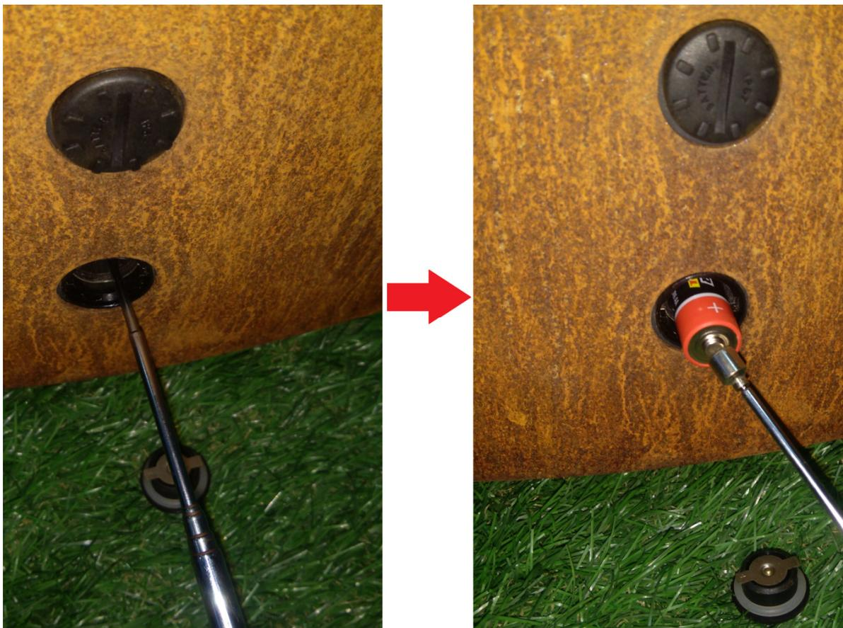
*Photo 7: Removing the second battery from the container*
