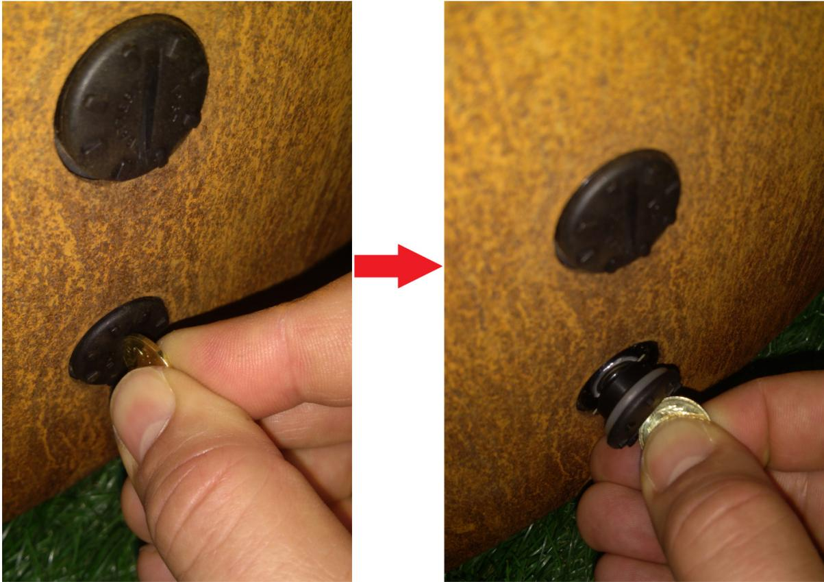
*Photo 5: Cover of the batteries container*
