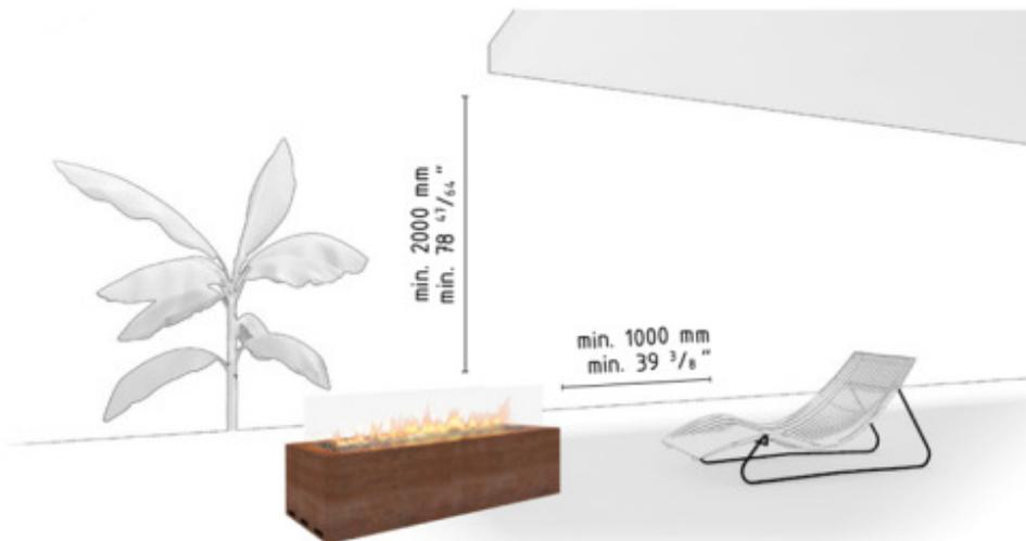
Figure 1: Minimum distance to flammable materials
