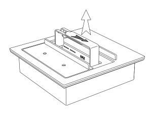
When the flat ends of the Lifting Handles are all the way inside the Combustion Chamber, slide the handle into the open position as far as it will go. Grip the handles Parts A and Part B firmly with one hand in the fully open position, then lift and insert the Combustion Chamber inside the Mount Plate.
