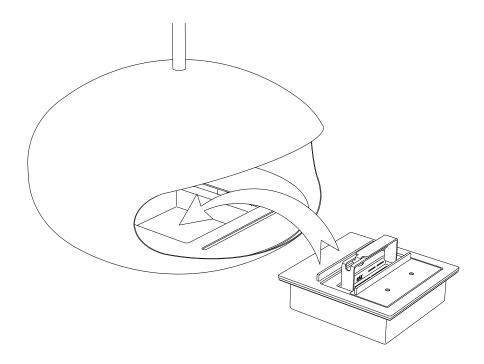
With the Mount Plate in the correct position and secured in place with the hex nut, the Combustion Chamber can now be placed inside and taken off the Mount Plate opening using the Lifting Handles supplied as shown on the previous pages.
