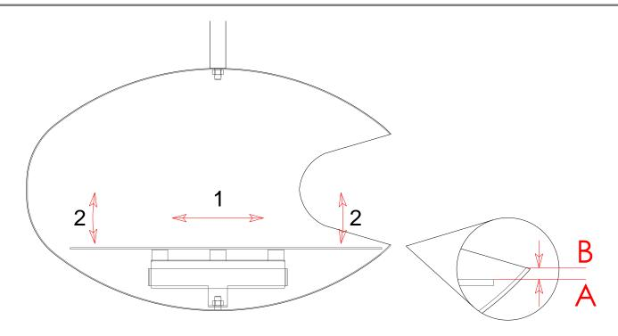
By finely adjusting the Removable Tray Bracket backward and forward (1) allows for the necessary adjustment in height (2) of the Mount Plate.
