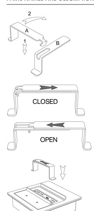
The Lifting Handle is used to take the Combustion Chamber in and out of the Mount Plate inside the Main Body for filling and cleaning. Step 1 is to join Part A and Part B as shown to the left. Once you have placed the tag of Part A into the slot of Part B, then twist it 90 degrees to lock them as one handle.
