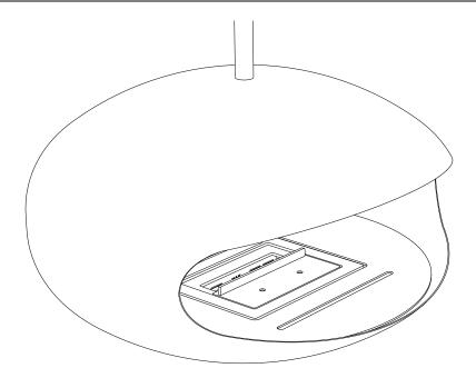
Once all spilled or residual fuel has been wiped clean, and all other forms of fuel have been sealed and moved to a safe distance from the Combustion Chamber, and the Combustion Chamber has been placed back inside the Chimenea as indicated above, it is safe to consider igniting the Combustion Chamber.
