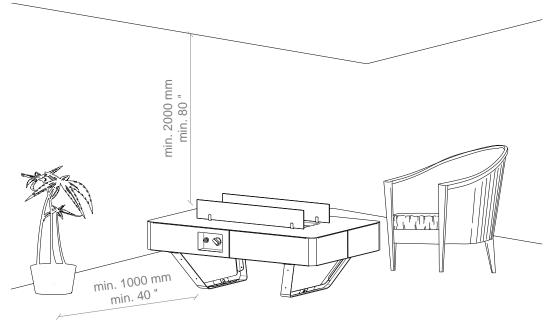
Fig. 1: Minimum distance to flammable materials
