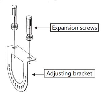
Step 5: Installation of two adjusting brackets; make sure lock brackets tight by butterfly hand screw.
