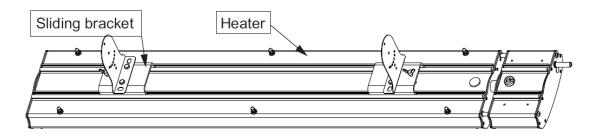
Step 4: Fix adjusting bracket into the wall by expansion screws.
