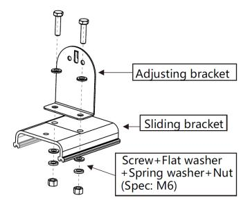
Step 3: Installation of sliding bracket & heater, as arrow points.
