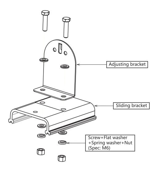
Step 3: Installation of sliding bracket & heater, as arrow points.
