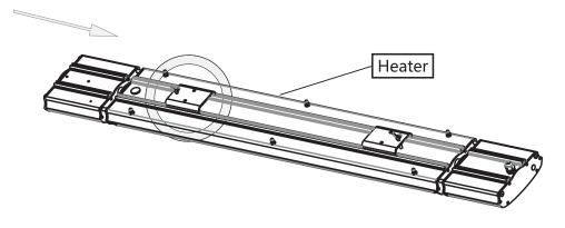
Step 4: Fix adjusting bracket into the wall by expansion screws.
