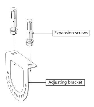
Step 5 : Installation of two adjusting brackets; make sure lock brackets tight by butterfly hand screw.
